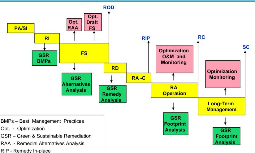
Figure 1. ER Process phases with Optimization Evaluations and GSR Analysis.
