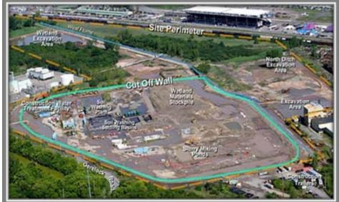
Remedy included greater risk waiver, slurry wall, pump-and-treat system, excavation of shallow soils, temporary cap, and long-term monitoring
