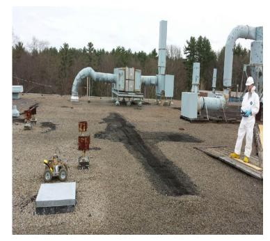
A remotely operated, GPS enabled, 2x2 sodium iodide survey instrument in use.
