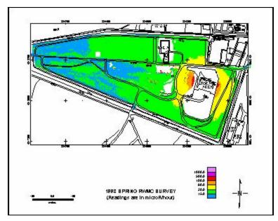
Figure C-1. Example of the Spring RWMC Survey Results
