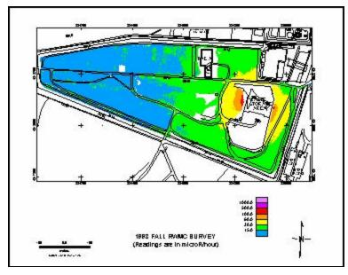
Figure C-2. Example of the Fall RWMC Survey Results
