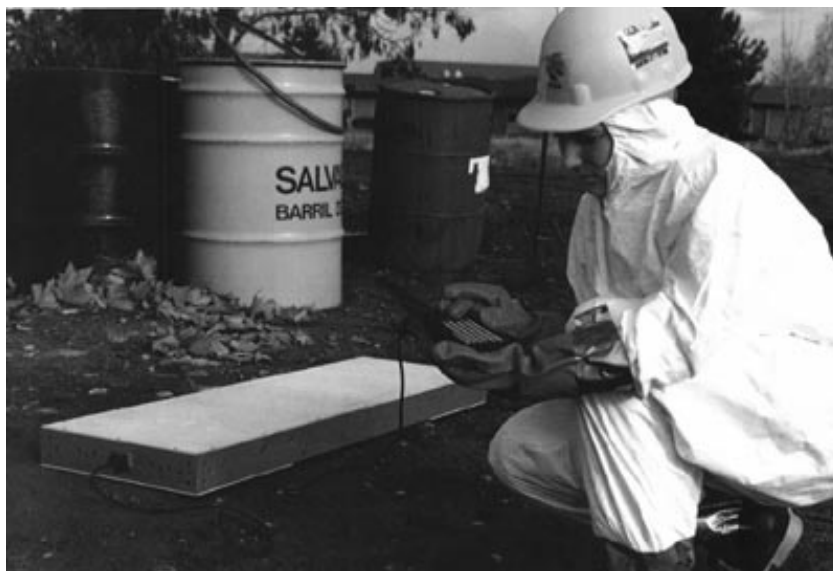
Figure 1B - The BetaScint™ surface/soil monitor can also be placed directly on or above contaminated soil or surfaces to detect and quantify radiation associated with the decay of U-238 or Sr-90. The instrument is roughly 1.5 m by 35 cm by 8 cm and weighs approximately 20 kg (excluding power supply).
