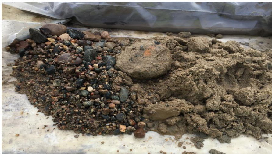
Photo 6: Contact between the Lower Gravel and the Upper Sand (Test Area 2)
