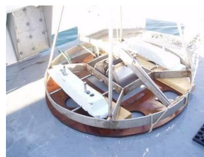
Figure 10-3. Sediment Sampling Using a 0.1 m 2 Van Veen Grab Sampler (Photo Courtesy of Battelle Ocean Sciences Laboratory)
