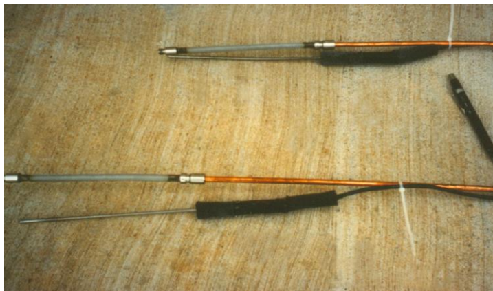
Figure 11-1. Example Permanent Soil Vapor Probes Constructed with Copper Tubing and Stainless Steel Screen (Source: Seminar on Indoor Air Vapor Intrusion, USEPA, 2003)
