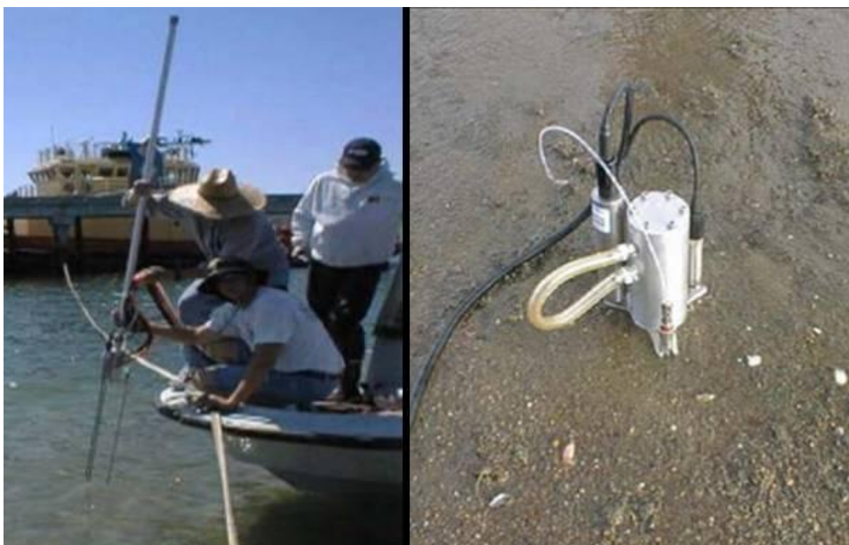
Figure 8-3. Trident Probe Prior to Inserting into Sediment (left); Top of Trident Probe after Placement in Sediment (right); (Source: RITS on Coastal Contamination Migration Monitoring, NAVFAC ESC, 2003)
