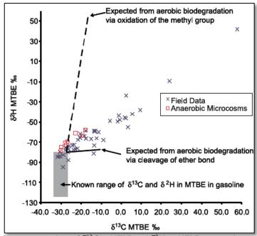
Concurrent analysis of  $\delta^{13}C$  in MTBE and  $\delta^2H$  in MTBE in groundwater to associate natural biodegradation of MTBE in groundwater with an anaerobic process that allows the selection of an appropriate value for the enrichment factor ( $\epsilon$ ) used to estimate the extent of biodegradation of MTBE<sup>5</sup>
