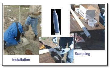
Photo of installation of passive flux meter (above). How flux meter works (right). (Photos courtesy of Enviroflux).
