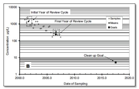
Example of MNA performance monitoring record over the interval of time in a review cycle<sup>12</sup>. At the end of the review cycle, data should be evaluated to determine whether attenuation is adequate to attain the long-term goal by a specified date.
