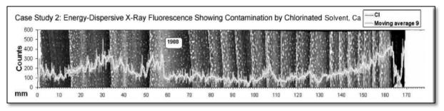
Cl patterns (shown on y-axis as x-ray fluorescence counts) over time in tree core (shown on x-axis in mm of core). Pattern identifies potential exposure events (releases) in 1988 and 1993/1994, along with continuing impact at date when core was collected (far right hand side)<sup>117</sup>
