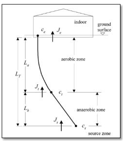
Conceptual Model for Vadose Zone Oxygen-Limited Biodegradation<sup>161</sup>
