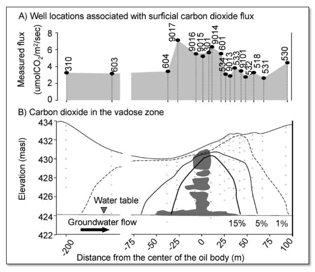
Surficial  $CO_2$  efflux from a series of wells located above a crude oil spill measured using the Dynamic Closed Chamber method<sup>33</sup>. Lower panel shows  $CO_2$  contours with depth within the same area.
