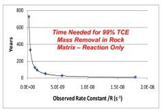
Impact of Observed Abiotic Degradation Rates in Rock Matrix on Mass Reduction Timeframes. Data obtained in study described in Schaefer et al. <sup>199</sup>
