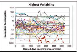
Range of variability between groundwater monitoring wells in 504-well, multiple year monitoring dataset from Hill AFB. Each graph shows 10% of wells with lowest, midrange, or highest variability from each data set. For each well, the contaminant concentration is normalized to the concentration measured during first monitoring event for that well.<sup>37</sup>
