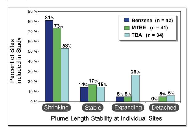
Results of groundwater plume stability analysis for MTBE, TBA, and Benzene at 48 site study<sup>49</sup>
