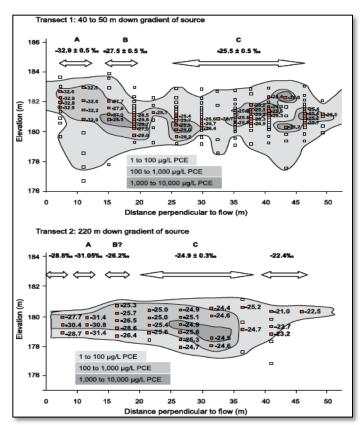
Concentrations and carbon isotope ratios of PCE in two transects downgradient of unidentified PCE sources. All values are given in % relative to the V-PDB standard. Filled squares are depths sampled for determination of both concentration and  $\delta^{13}C$ . Open squares are depths sampled for concentration only. The figure is modified after<sup>70</sup> (from <sup>5</sup>)
