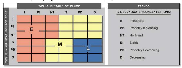
By entering the trend in the source zone wells on the rows, and the trend in the plume in the columns, a site is defined as either needing an Extensive (E); Moderate (M), or Limited (L) monitoring system. Almost all MNA projects would likely either be in the M or L categories.
