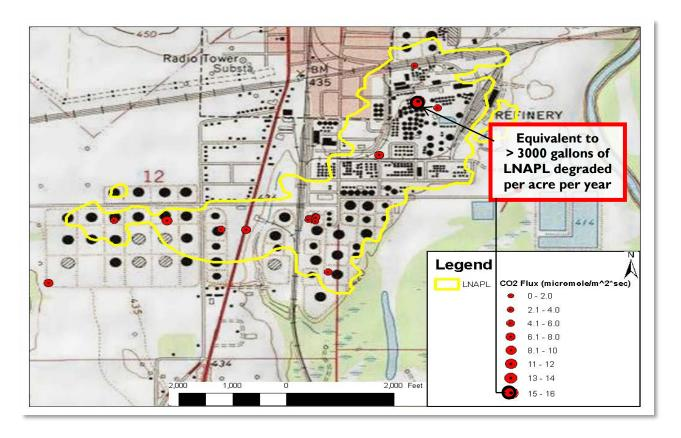
Example of field site where CO<sub>2</sub> traps were used to delineate LNAPL natural loss rates. <sup>121</sup>
