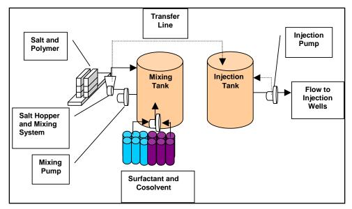
FIGURE 4-2. Schematic of Surfactant/Cosolvent Injection System
