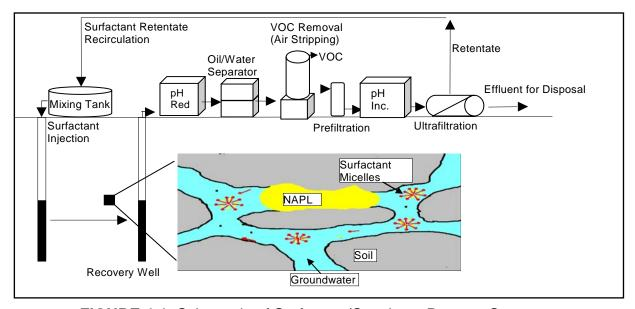
FIGURE 4-1. Schematic of Surfactant/Cosolvent Process System
