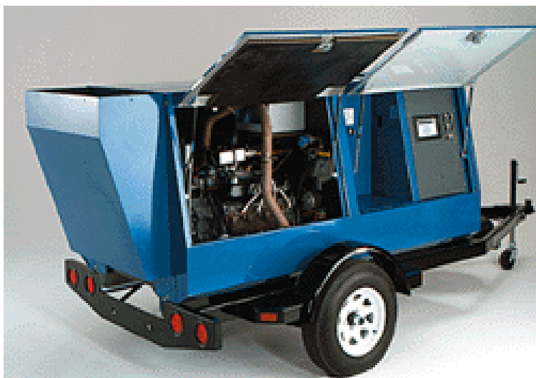
Figure 3-6. Internal Combustion Engine Remediation System
