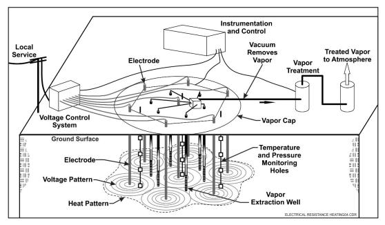
Electrical Resistance Heating System Schematic
