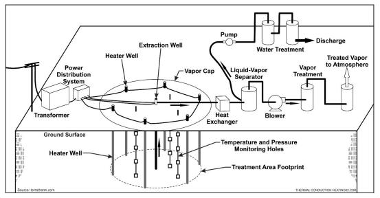
Thermal Conduction Heating System Schematic
