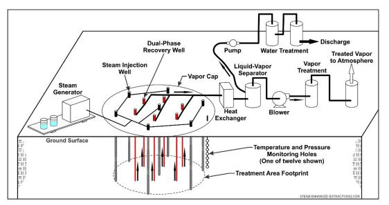
In Situ Steam Flooding Heating System
