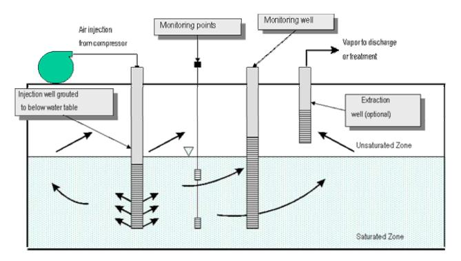
Figure 1. Schematic Diagram of a Typical Air Sparging System.
