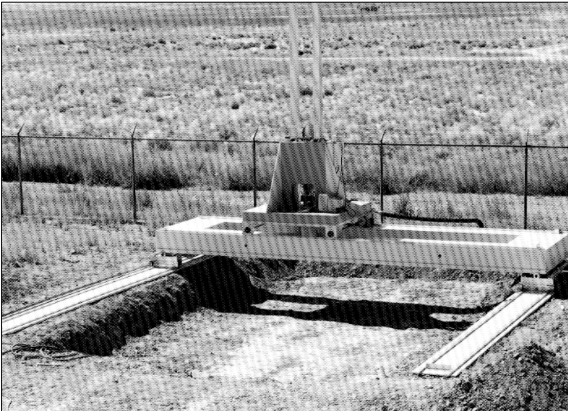
Figure 5. Photograph of trolley during full-function testing at the INEEL Water Reactor Research Test Facility
