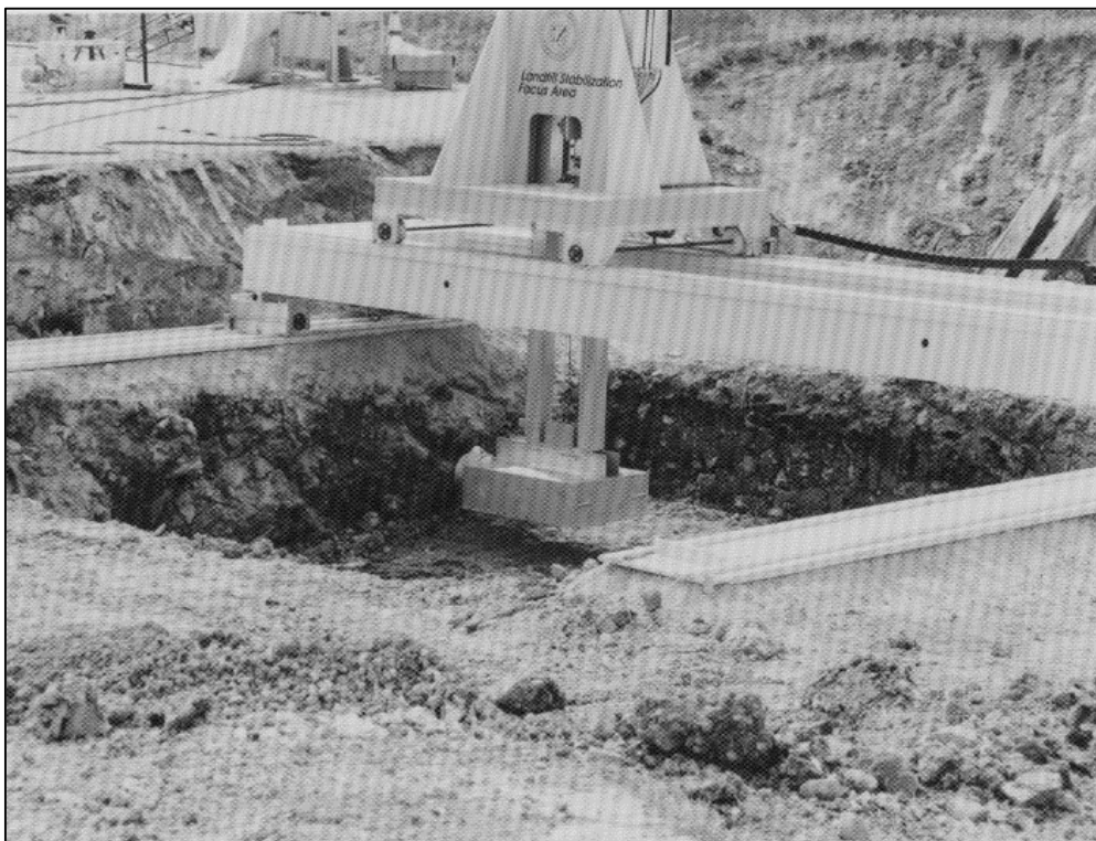
Figure 2. Gamma/neutron mapper mounted on trolley
