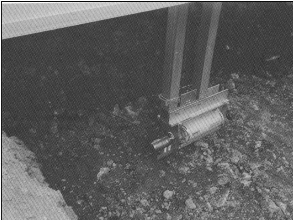
Figure 3. Ge-spectrometer mounted on the trolley
