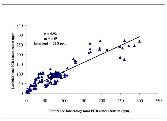
Figure 2. L2000DX PCB results versus reference laboratory results for all samples.
