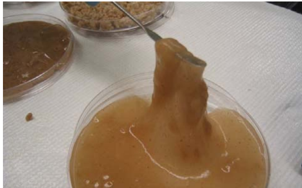
Adhesive product of sand coated with guar crossed with borax
