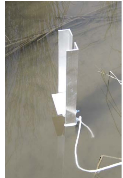
Depth profiling of porewater in sediment
