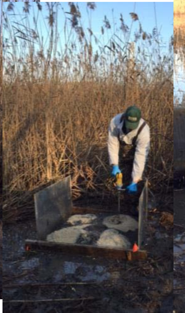
Buckets of pre-measured sand-chitin-seeded GAC dumped in plot and mixed into sediment to depth of 10 inches with small auger or “egg-beater” attachments on drill.
