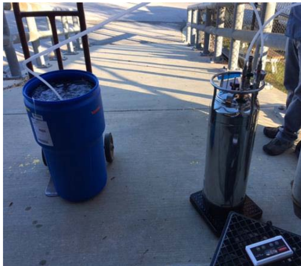
WBC-2 in anaerobic cylinder from Sirem Lab (20L mixed with DI-H 2 O for GAC seeding)
