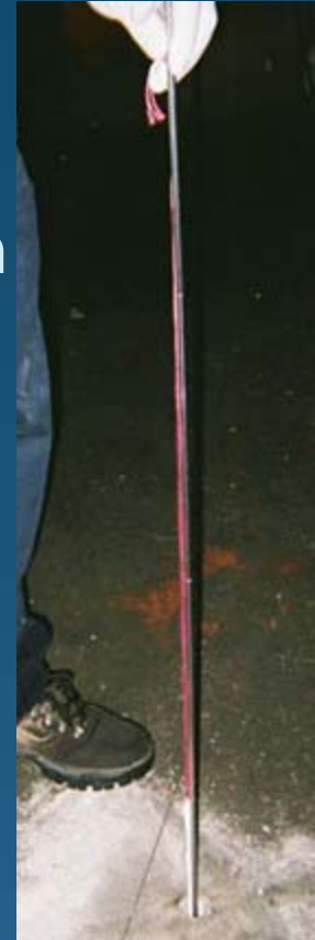
Passive sampler insertion
