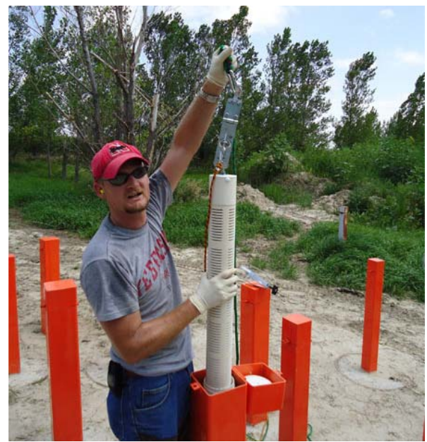
Mark Christenson shows how paraffin-based permanganate candles are prepped for lowering down a borehole at a Cozad landfill site.
