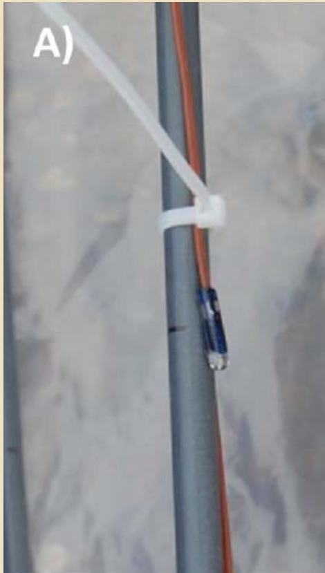
Thermocouple on temperature monitoring "stick."
