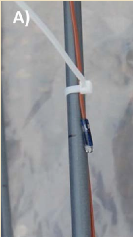
Thermocouple on temperature monitoring "stick."
