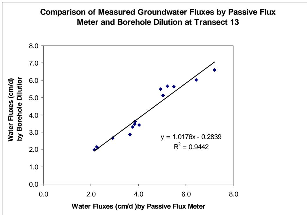
Figure 4-9. The comparison of measured groundwater fluxes inside a screen well by Passive Flux Meter and Borehole Dilution (BHD) during the second field test at CFB over the 13<sup>th</sup> sampling transect in the forested area (April 2002).
