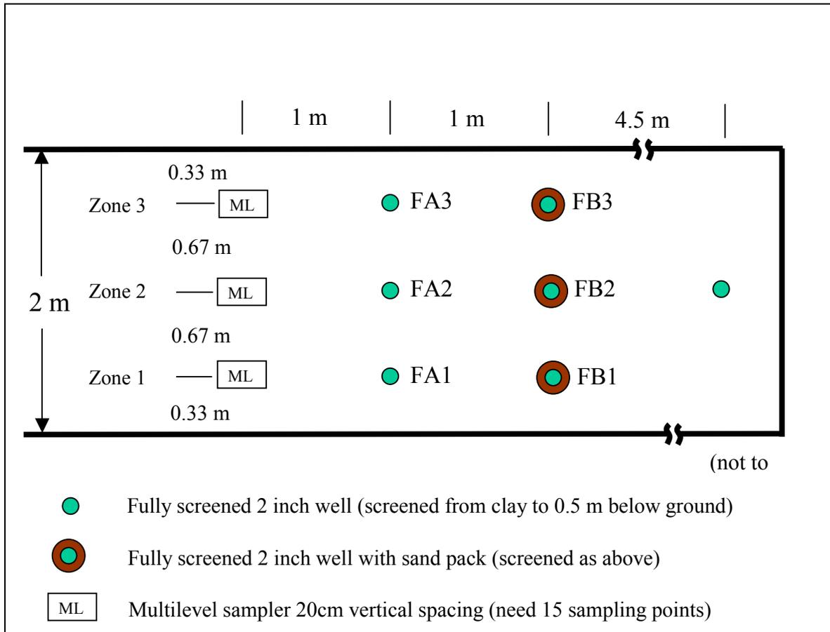
Figure 4-7. Subsurface gate (gate) facility.
