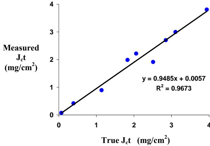
Figure 4-6. Measured cumulative DMP fluxes versus true fluxes.
