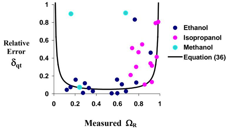
Figure 4-5. Absolute water flux prediction errors versus the relative mass of resident tracer remaining in the meter with equation (4-6).
