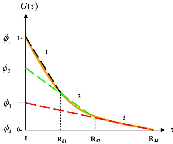
Figure 2-6. A hypothetical nonlinear resident tracer elution function,  $G(\tau)$  for a streamtube and three piece-wise linear segments shown with defining parameters  $\phi_i$  (for  $i = 1, \dots, 4$ ) and  $R_{di}$  (for  $i = 1, \dots, 3$ ).
