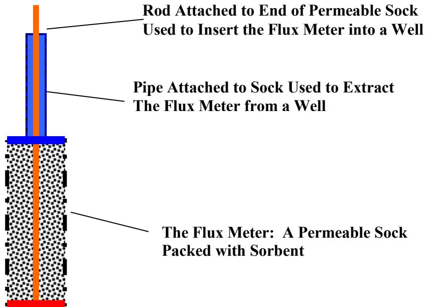
Figure 2-1. Schematic of a Flux meter comprised of a permeable sock filled with a selected sorbent.
