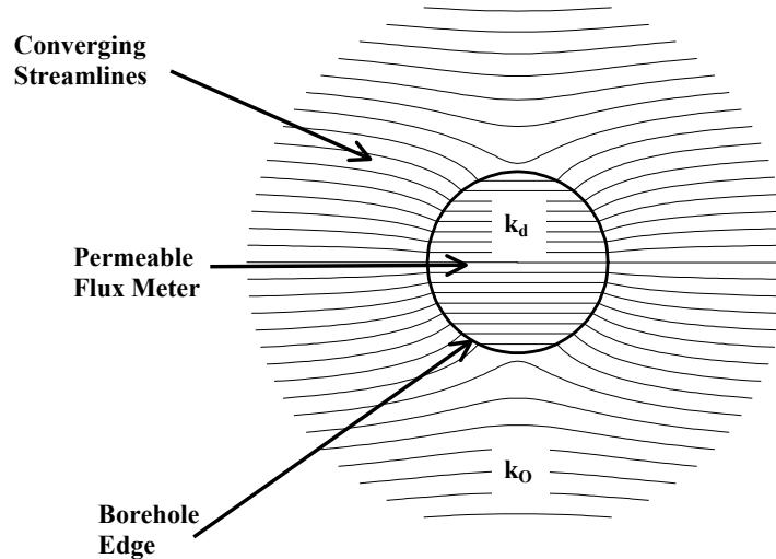
Figure 2-7. Groundwater streamlines through a flux meter where the conductivity of the meter  $k_d$  is greater than that of the surrounding aquifer,  $k_o$ .
