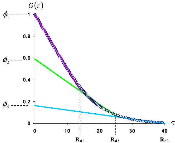
Figure 4-1. The actual nonlinear ethanol resident tracer elution function,  $G(\tau)$  from a column experiment [open circles] and three piece-wise linear segments shown with defining parameters  $\phi_i$  (for  $i = 1, \dots, 4$ ) and  $R_{di}$  (for  $i = 1, \dots, 3$ ).
