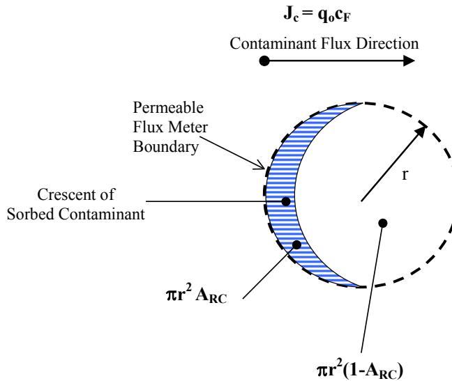
Figure 2-8. Conceptual model of how contaminant would be retained on the sorbent of a passive flux meter.
