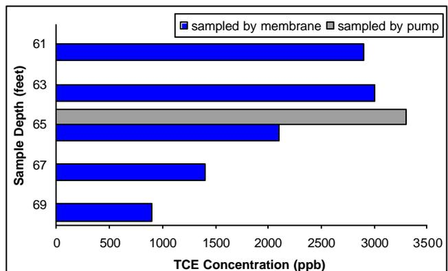
Figure 5 – Lab results comparing samples obtained by diffusion membrane and low-flow pumping
