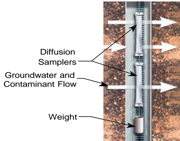
Figure 1 – Diffusion samplers placed at multiple depths to define vertical contamination profile
