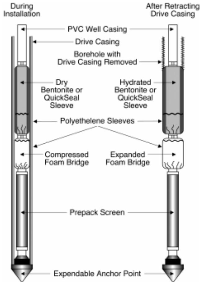
**Figure 2-2. Example of protected-screen Direct Push well installation.**
