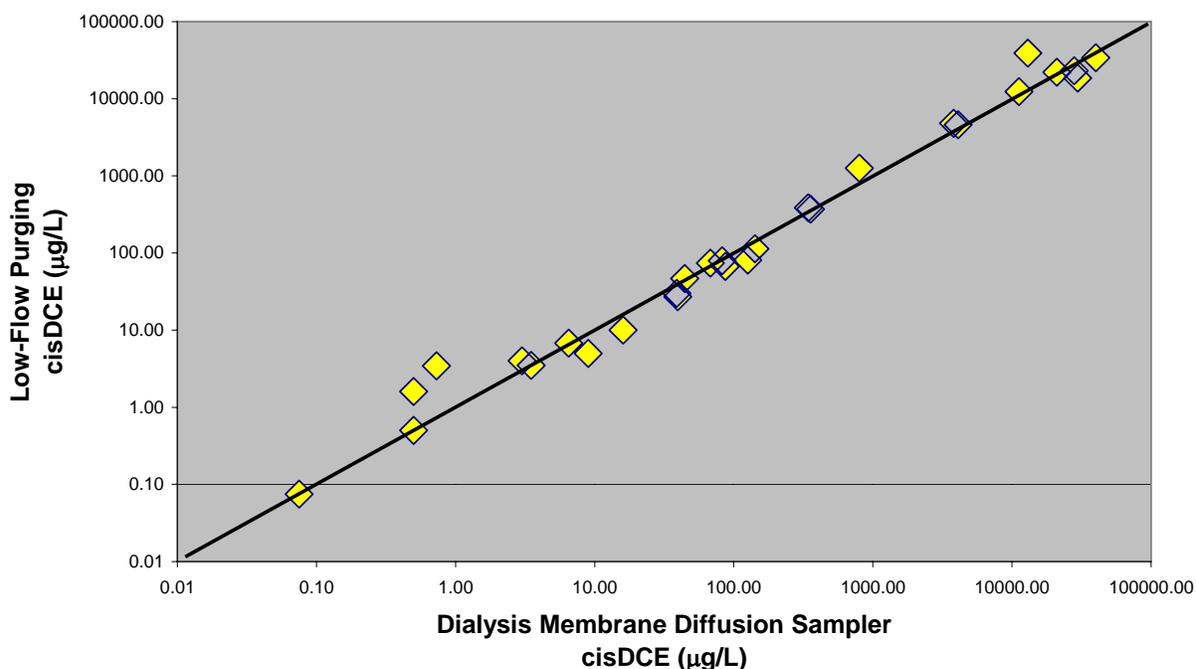
**Figure 5-6. A 1:1 correspondence plot comparing *cis*-1,2-dichloroethene results in dialysis sampler and low-flow purging samples from wells at the Naval Air Warfare Center, West Trenton, New Jersey, 2000–2002. (Sources: Imbrigiotta et al. 2002 and Imbrigiotta, unpublished data)**
