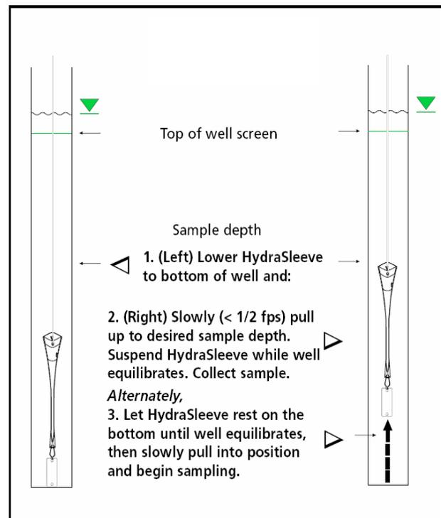
Figure 3-4. Bottom-up deployment.
