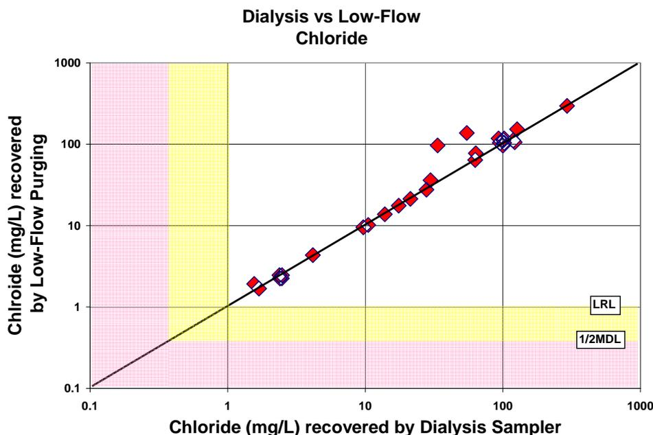
**Figure 5-8. A 1:1 correspondence plot of dialysis sampler vs. low-flow purging results for chloride. LRL = lower reporting limit; 1/2MDL = one-half minimum detection limit. (Source: Source: Imbrigiotta, Trotsky, and Place, forthcoming)**
