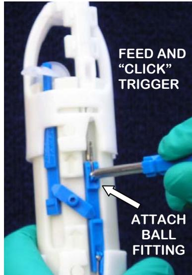
**Figure 4-6. Feeding and securing trigger cable.**
