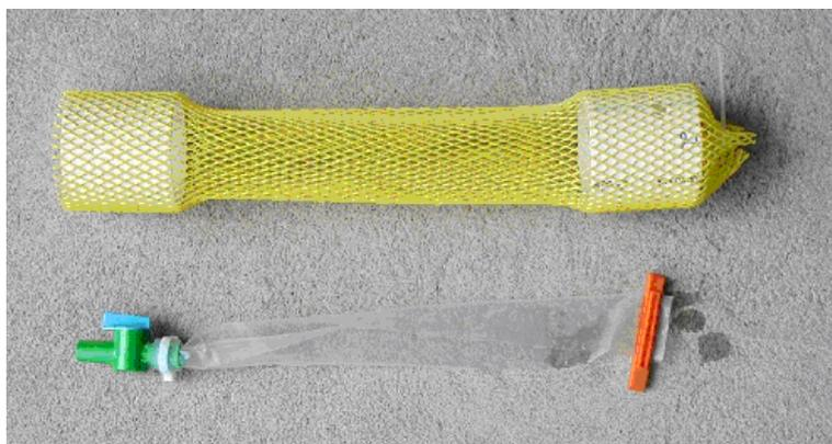
**Figure 5-3. Partially assembled dialysis sampler before filling with deionized water with external supports installed in the protective mesh.**
