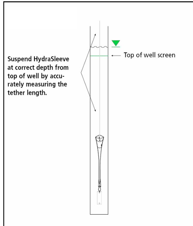
Figure 3-3. Top-down deployment.
