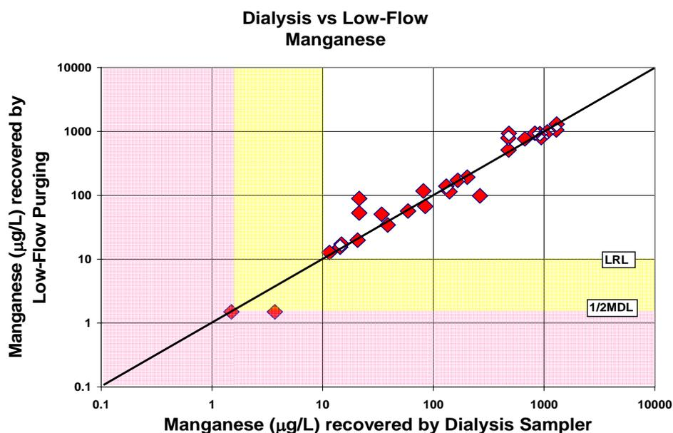
**Figure 5-7. A 1:1 correspondence plot of dialysis sampler vs. low-flow purging results for manganese. LRL = lower reporting limit; 1/2MDL = one-half minimum detection limit. (Source: Imbrigiotta, Trotsky, and Place, forthcoming)**
