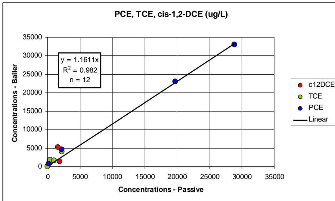
**Figure 2-8. Comparison of the chlorinated compounds observed in monitoring wells at a dry cleaner.** The concentrations on the x-axis were calculated and compared to the measured concentrations (y-axis).
