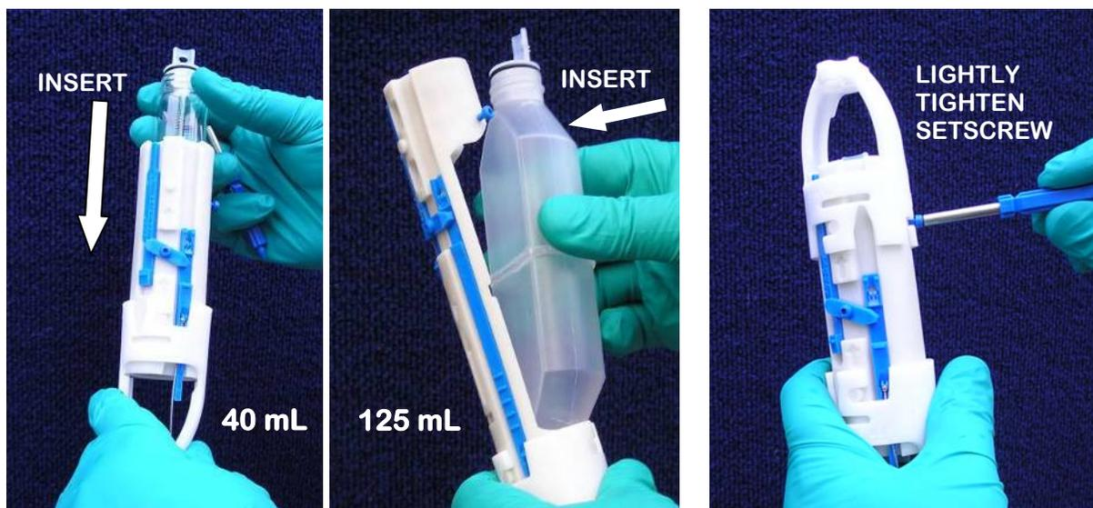
**Figure 4-3. Inserting sample bottles into Snap Sampler bodies.**
