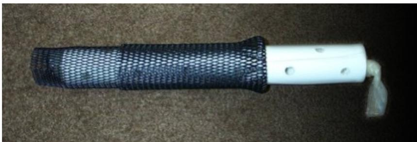
**Figure 5-5. Dialysis sampler with rigid perforated support internal to the dialysis membrane.**
