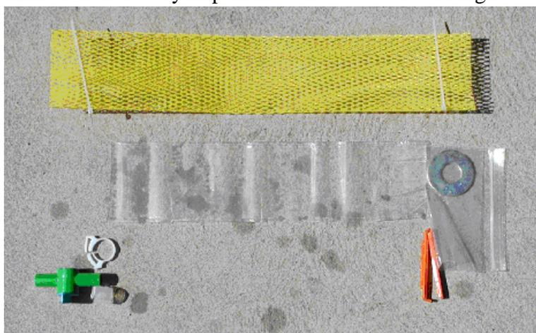
**Figure 5-2. Parts of a dialysis sampler before assembly.**
