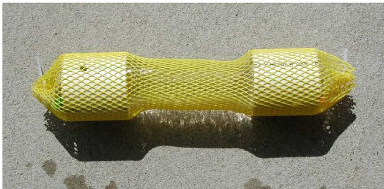
**Figure 5-4. Fully assembled dialysis sampler with supports external to the dialysis membrane.**
