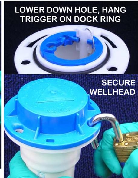
**Figure 4-7. Securing sampler into wellhead docking station.**
