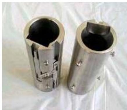
**Figure 4-1. Snap Sampler body.**
