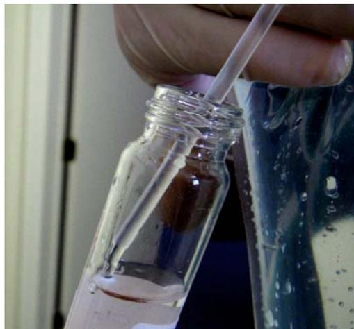
**Figure 3-11. Discharging sample from HydraSleeve.**
