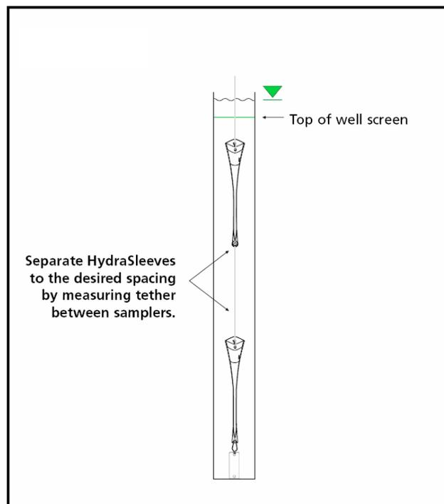
**Figure 3-7. Multiple samplers attached end to end.**
