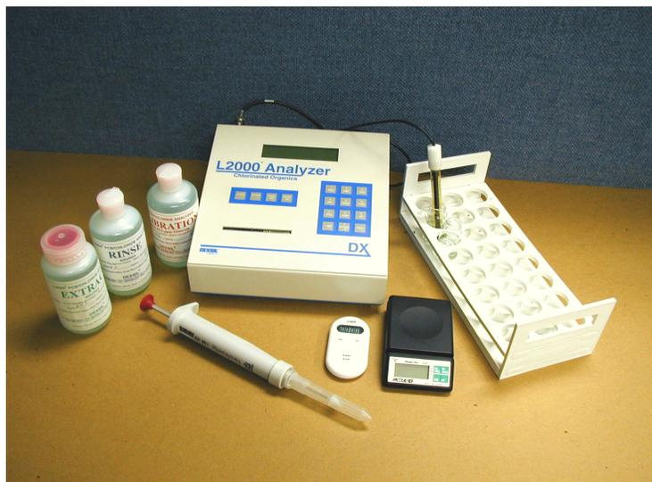
Figure 1. L2000DX Analyzer.
