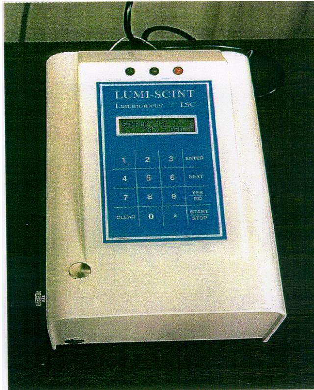
Figure 1. Lumi-Scint portable liquid scintillation counter.
