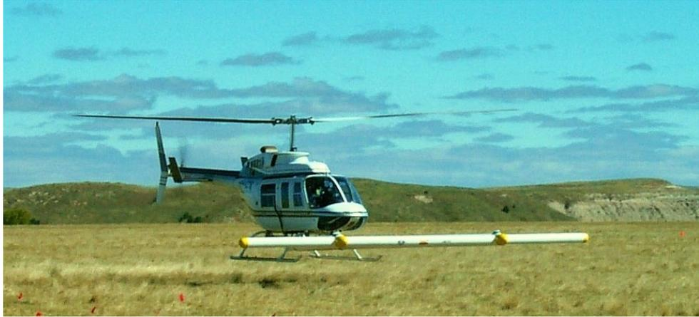
**Figure 7-8. NRL Airborne MTADS magnetometer system.**
