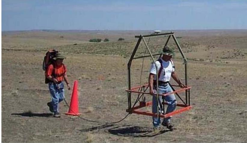
**Figure 3-19. Man-portable platform.**
