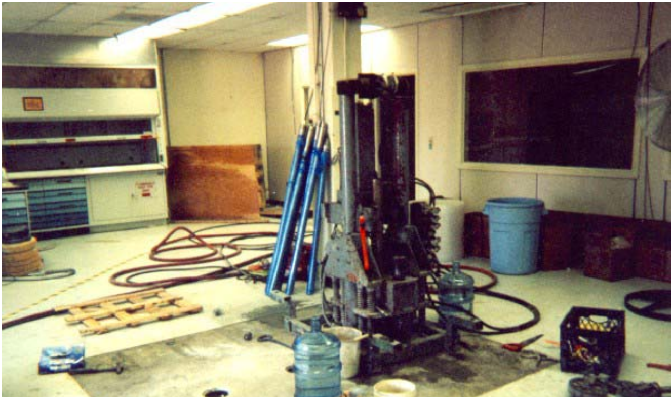
Figure 4-5. Indoor Vibra-Push Rig (LD Geoprobe® Series) Used in the Engineering Support Building
