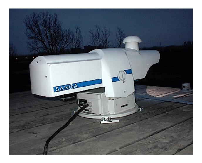
Figure 1. UV-DOAS Projector on the roof of Trailer #2.
