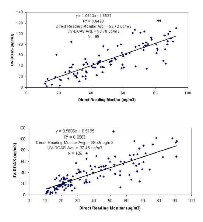
Figure 9. Direct reading and UV-DOAS nitrogen dioxide concentrations (A) nighttime, 1900 to 0500 hours, (B) daytime, 0600 to 1800 hours.
