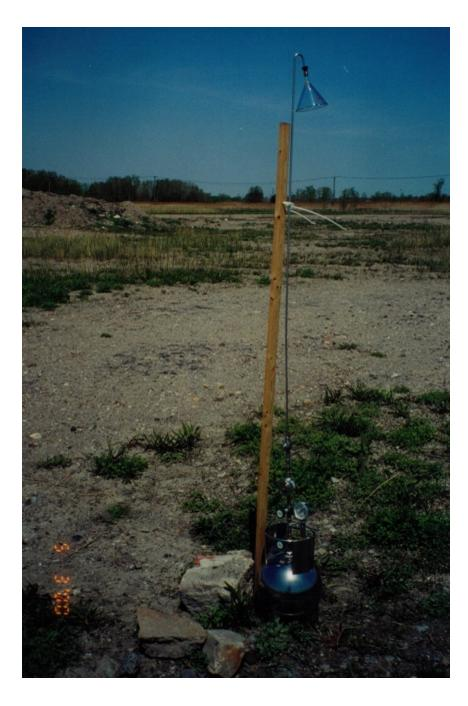
Figure 6. VOC Canister Sample.
