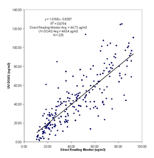
Figure 8. Comparison of direct reading and UV-DOAS nitrogen dioxide concentrations.
