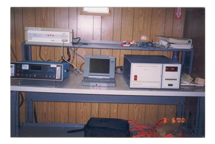
Figure 5. TECO 42 NOx Monitor (on the right) and Dasibi Model 1003AH Ozone Monitor (on the left) inside Trailer # 2.
