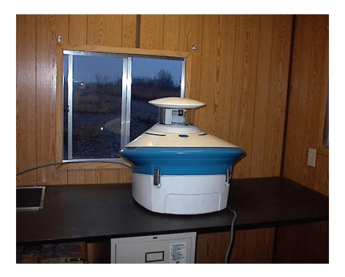
Figure 2. UV-DOAS Receiver inside Trailer #1.
