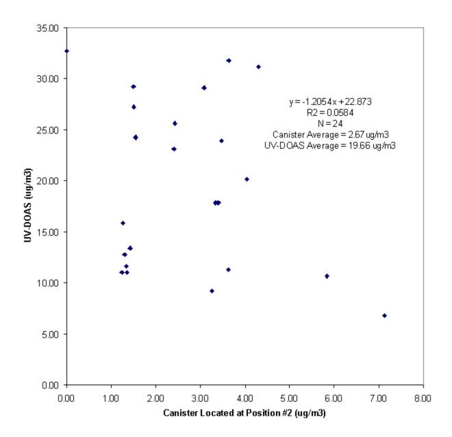
Figure 17B. Benzene concentrations: UV-DOAS data versus data obtained from canisters located in Position 2.
