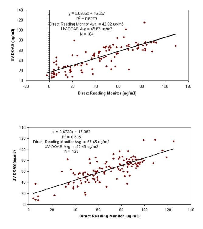
Figure 10. Direct reading and UV-DOAS ozone concentrations, (A) nighttime, 1900 to 0500 hours, (B) daytime, 0600 to 1800 hours.
