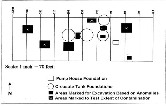
Figure 8: Locations Selected For Screening by Geophysical Surveys [1]
