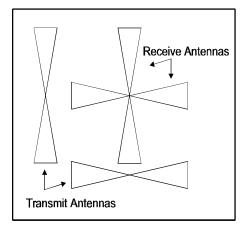
Multi-component GPR antenna arrangements
