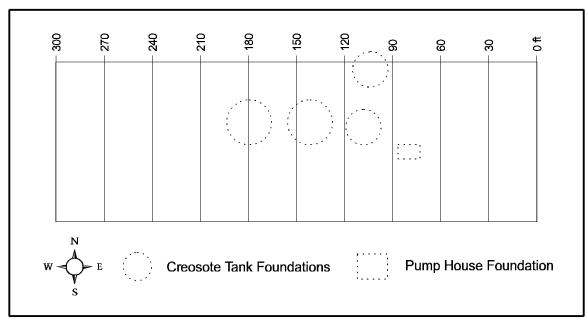
Figure 4: Geophysical Survey Area Showing North-South Traverse Lines [1]
