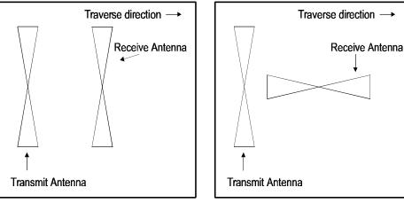
Co-pole perpendicular to traverse direction
