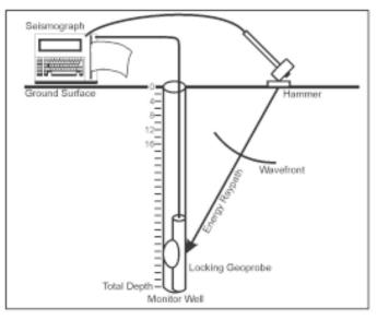
Figure 1. Vertical seismic profile schematic.
