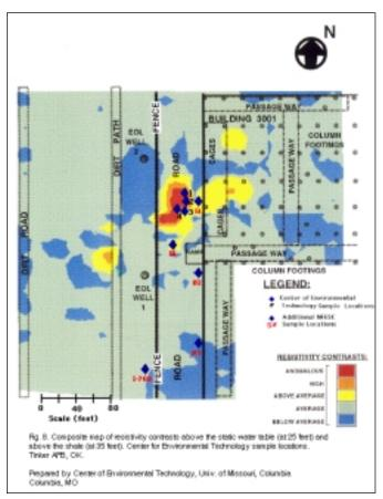
Figure 7. Composite map of resistivity contrasts.
