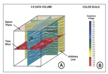
Figure 3. 3-D data volume schematic and seismic plot.
