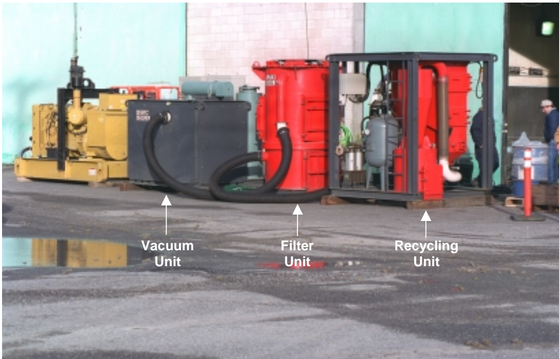
Figure 3. En-vac Blasting System
