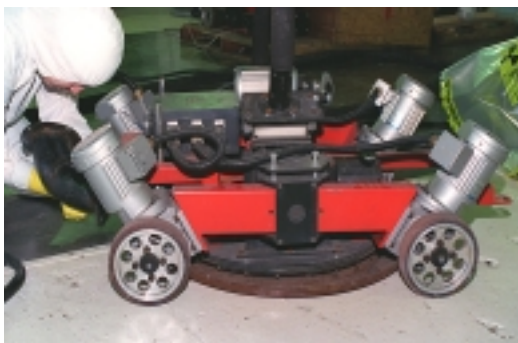
Figure 1. En-vac Robotic Wall Scabbler
