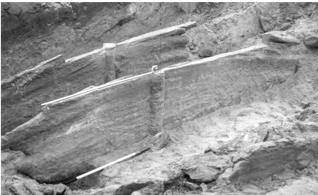
Figure 1. Photograph of thin-diaphragm walls emplaced by using high-pressure jetting.
