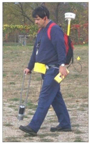
Figure 4. Gamma walkover equipment with GPS.
