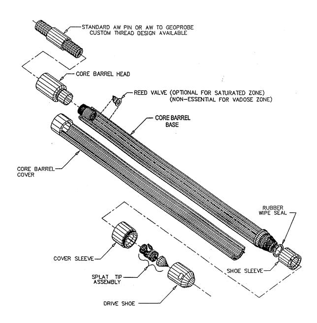
Figure 2-1. Core Barrel Assembly (Simulprobe®, 1997)
