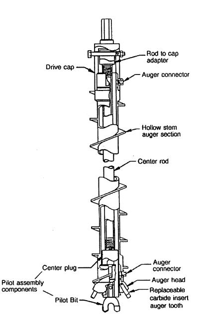
Figure 4-2. Typical Components of a Hollow-Stem Auger (Central Mine Equipment Co., 1994)
