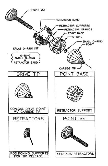
Figure 2-2. SPLAT<sup>™</sup> Assembly Discrete Sampling Mode (SimulProbe<sup>®</sup>, 1997)
