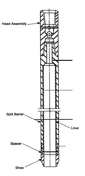
Figure 4-1. Split-Spoon Soil Sampler (modified from Central Mine Equipment Co., 1994)
