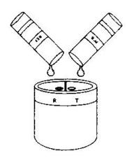
Figure 2-4. Filling the cup assembly.
