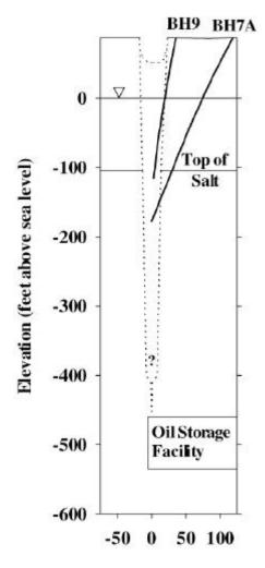
Figure 7. Cross section through the SPR Weeks Island sinkhole.
