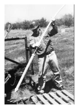
Figure 1. A flow sensor being installed through a hollow-stem auger.
