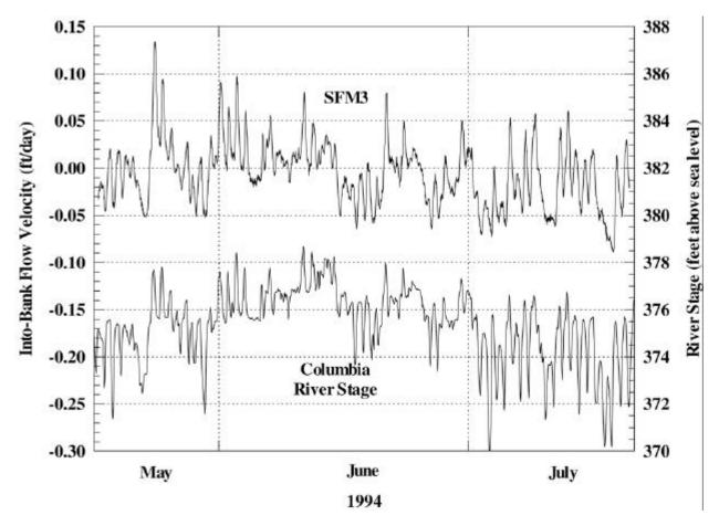
Figure 5. Columbia River stage (right vertical axis) and into-bank component of horizontal flow velocity (left axis) measured by flow sensor SFM3 during first data collection interval.
