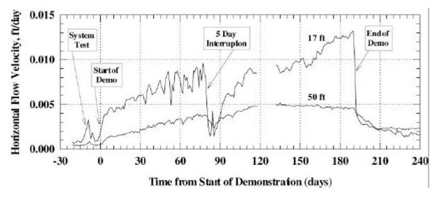
Figure 6. Horizontal flow velocity, relative to background, recorded by the near and far flow sensors during a demonstration at Edwards Air Force Base.
