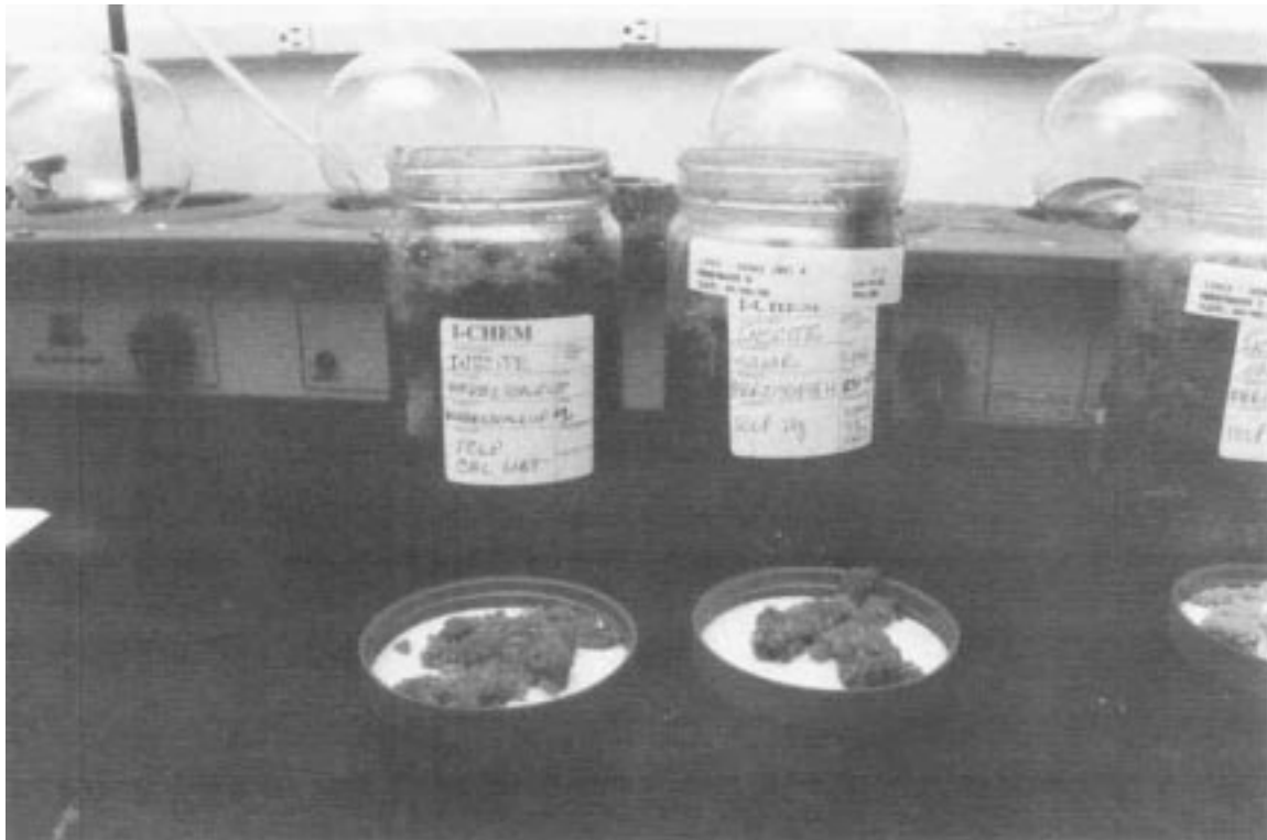
Figure 5. Comparison of waste treatment products from Allied Technology Group stabilization process: demonstration (left) and bench test (right) results.
