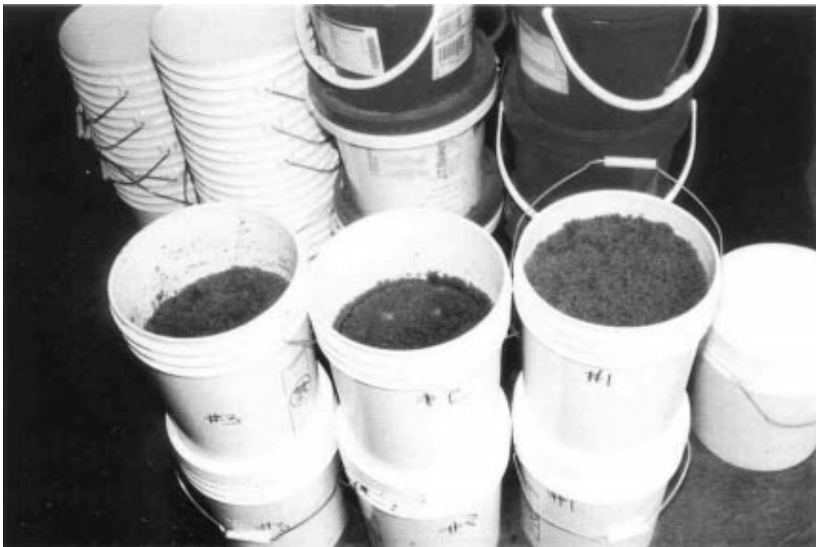
Figure 4. Six numbered pails containing all treated waste from demonstration of the Allied Technology Group stabilization process.
