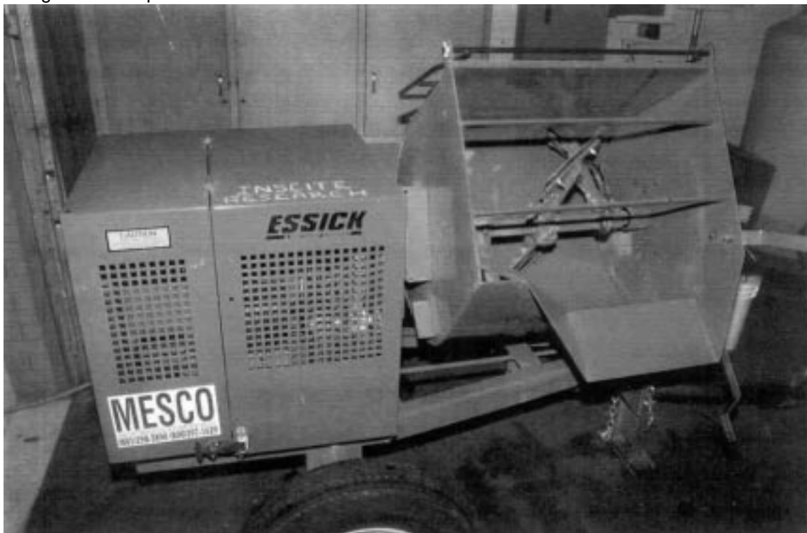
Figure 1. Mortar mixer used in Allied Technology Group process for stabilization demonstration.
