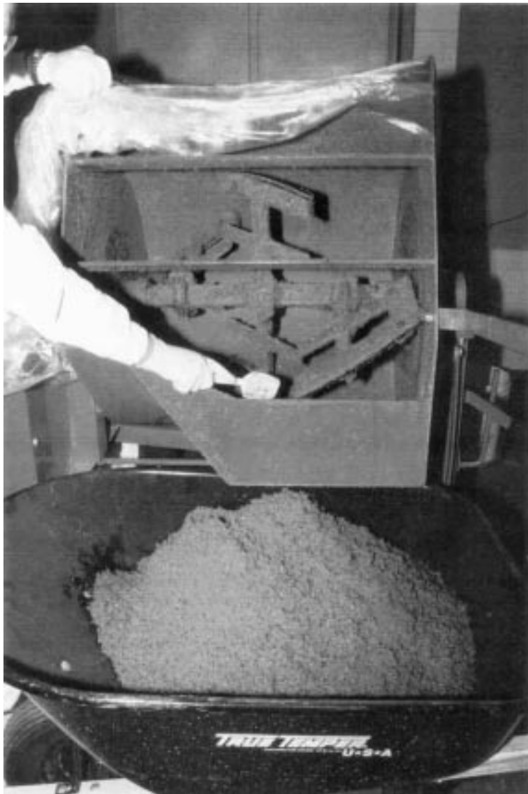
Figure 2. Emptying mortar mixer during Allied Technology Group demonstration of MER02 stabilization process.
