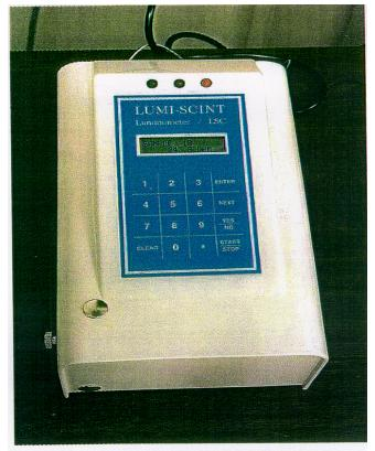
Figure 1. Lumi-Scint portable liquid scintillation counter.
