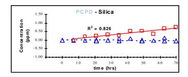
Figure 9. Silica Flux for Good Chamber Seal
