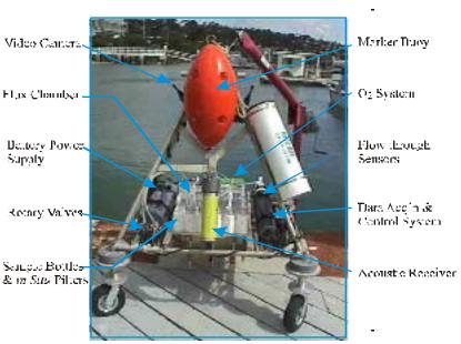
Figure 1. Benthic Flux Sampling Device 2
