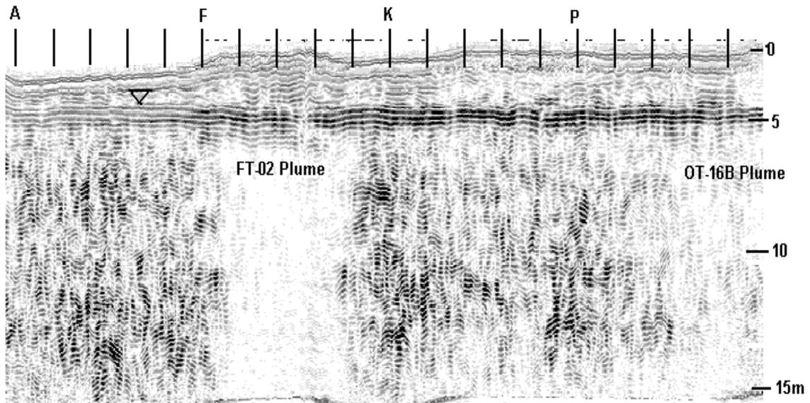
**Figure 2: Ground penetrating radar profile of Line 14 showing the strong amplitude shadow caused by the proximal end of the neighboring FT-02 plume, and the somewhat weaker shadow at the right end caused by the OT-16b plume. Source: [8]**
