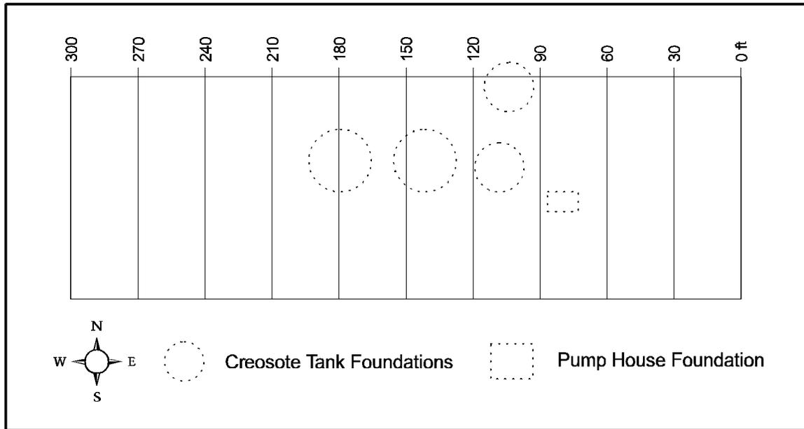
**Figure 4: Geophysical Survey Area Showing North-South Traverse Lines [1]**
