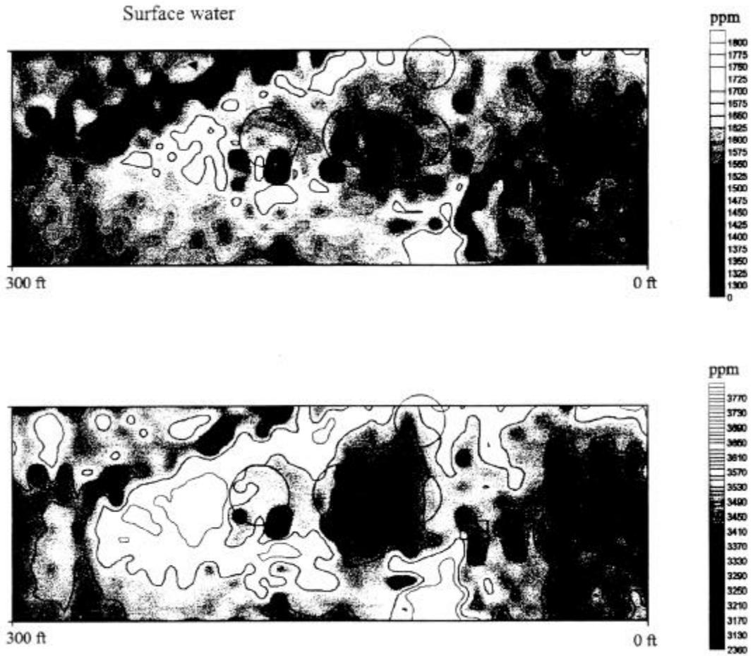
Figure 7: Electromagnetic Conductivity of Soils in Study Area [1]
