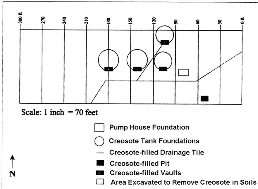
Figure 9: Locations of Significant Soil Contamination [1]
