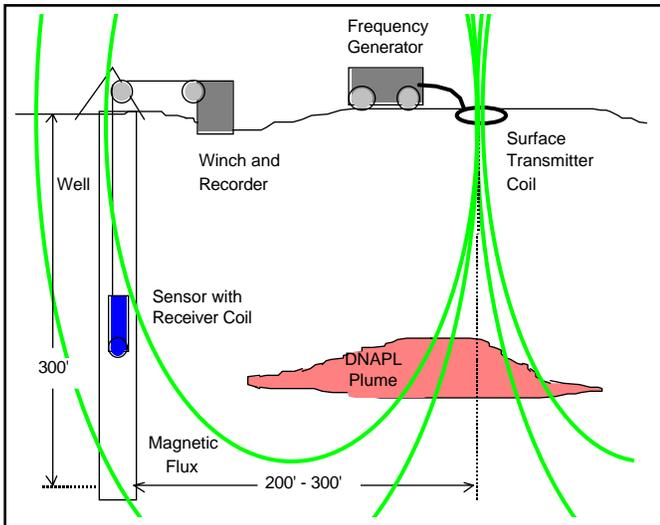
Figure 5. 3-D resistivity transmitter and receiver system.
