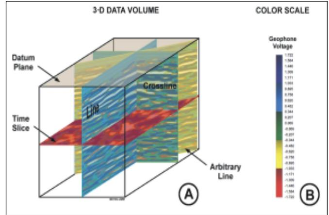
Figure 3. 3-D data volume schematic and seismic plot.
