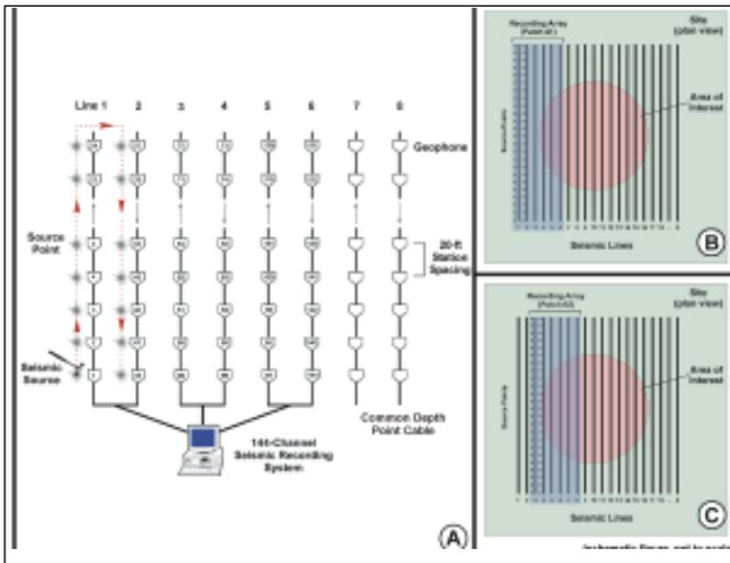
Figure 2. 3-D data acquisition schematic.
