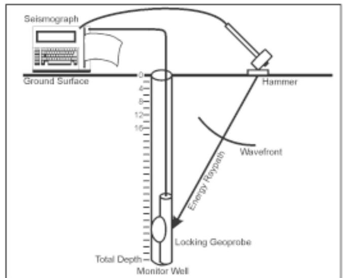
Figure 1. Vertical seismic profile schematic.
