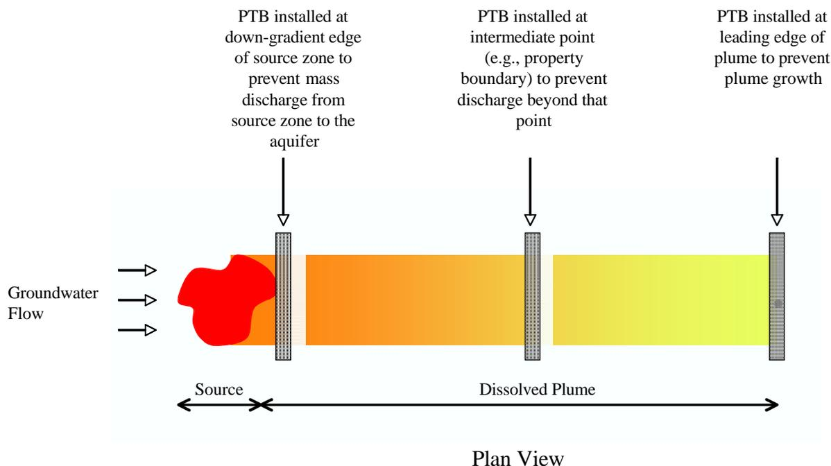
**Figure 1. Schematic of Deployment Options for PTBs.**
