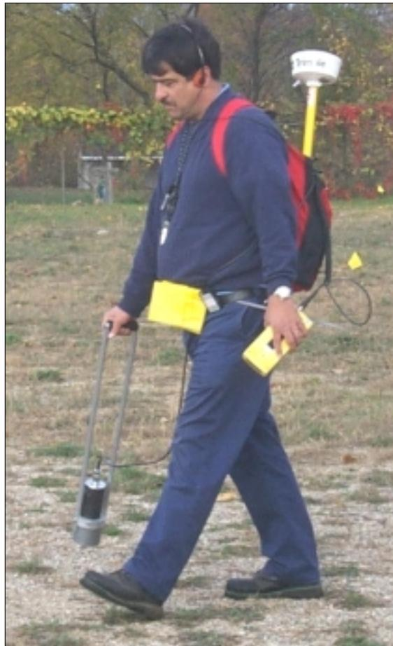
Figure 4. Gamma walkover equipment with GPS.
