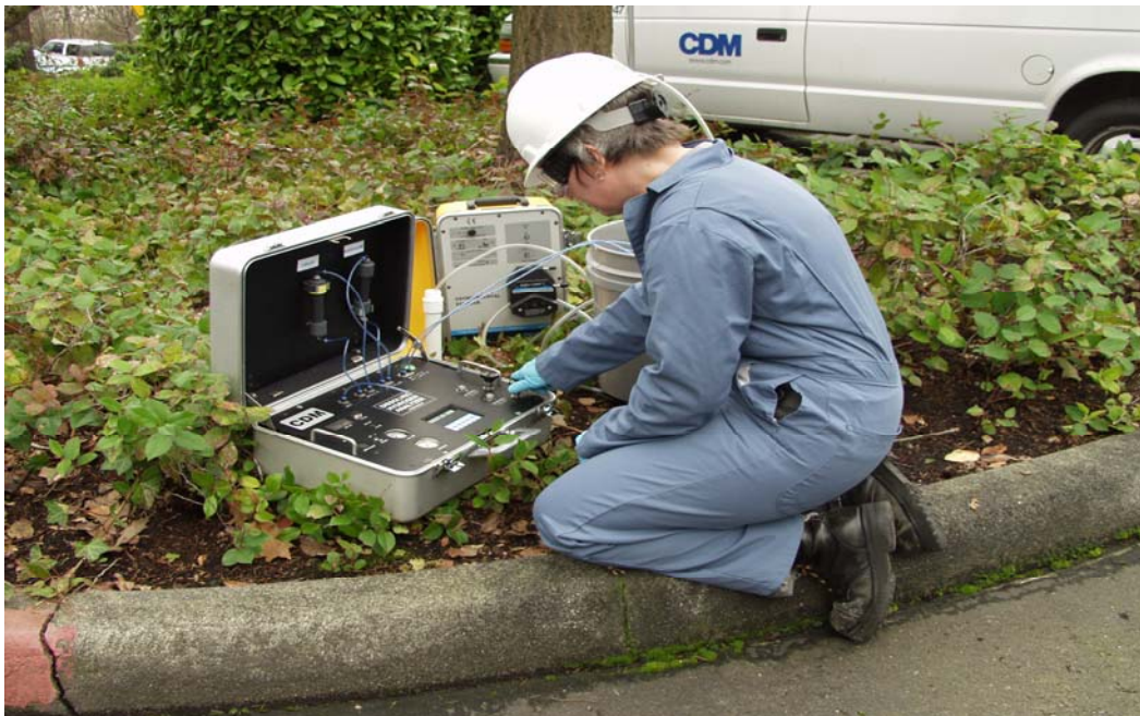
Figure 2-2. Dissolved Hydrogen Analyzer Implementation
