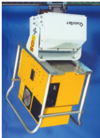
Figure 1. 3-D GammaModeler™ Sensor Head
