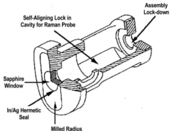
Figure 3. Sapphire window assembly.
