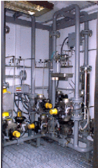
Figure 1. Endress+Hauser Promass 63M Coriolis meter installed in GAAT Slurry Monitoring Test Loop.
