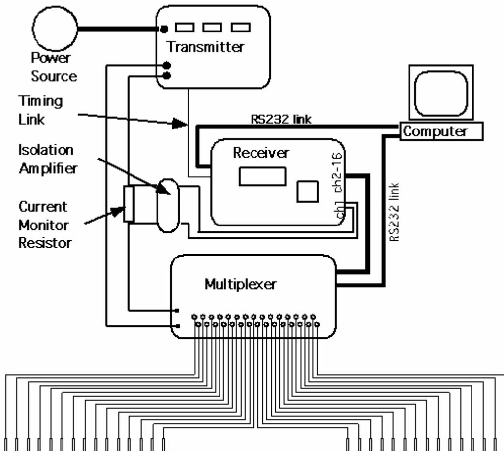
**Figure 2. Diagram of High-Speed Data Acquisition System Used in Electrical Resistance Tomography For Subsurface Imaging**
